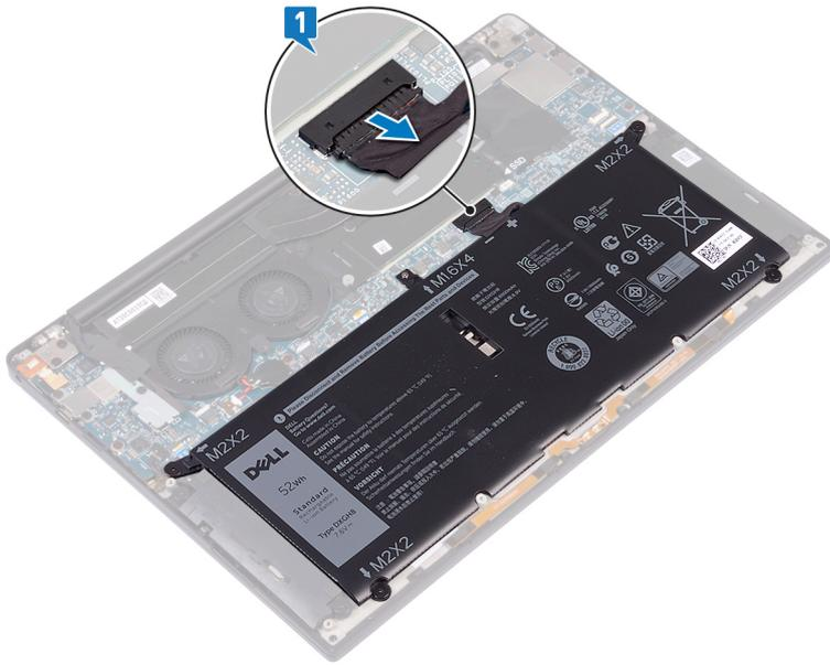
2. Remove the four screws (M2x2) that secure the battery to the palm-rest assembly.
